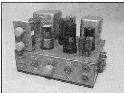
The Stancor ST-203-A with the cover removed.
