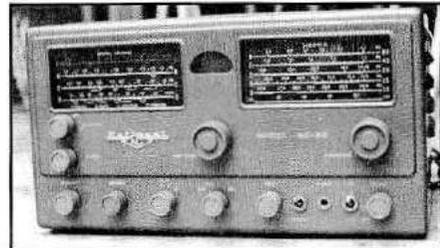
Figure 3—The National NC-98. Equipment with hammer-tone finishes such as this can be difficult to restore. Fortunately, this one's finish was in relatively good shape, requiring mostly clean-up to get it into the shape shown here.
