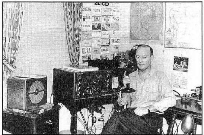
Bill's 1954 station: receiver NC-183D, transmitter behind his shoulder is a Stancor model 69. The BC-221 frequency meter was used as a VFO and also was used for ARRL frequency measuring contests and when Bill was an Official Observer.
