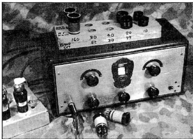
Figure A—Rationalized Autodyne, power supply and spare coils.
